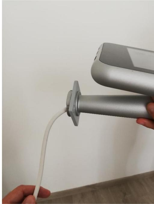
5. Connect the power supply and the network cable to the ScanFACE wiring
